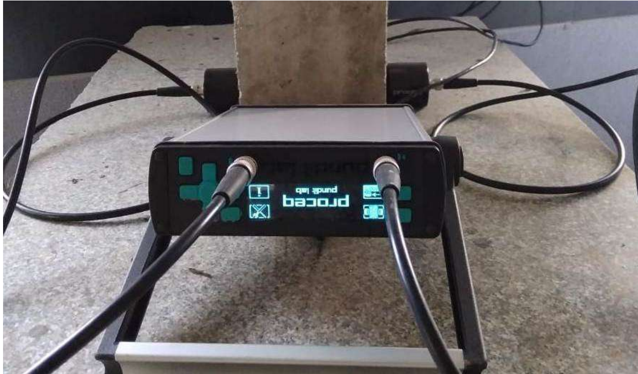
Fig.3 Ultrasonic pulse velocity measuring instrument and different techniques of pulse transmission .
